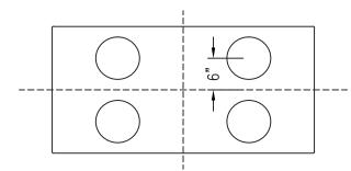
24" wide benches shall have (2) steel pedestals at each support point.
