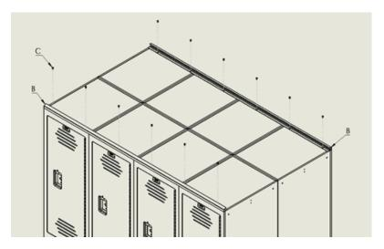
Pre-drill holes using a #19 drill bit .166" dia. x .44" deep in the locker top to acceptscrews (C)
