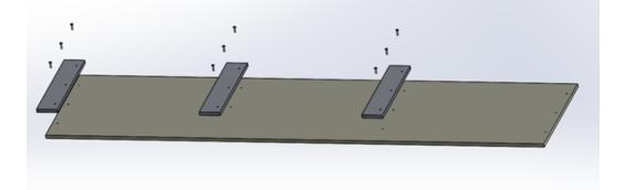
Depending on the direction that the slope tops are being installed one set of the brace holes **<u>may not be used</u>**. This is to account for the overlap of the adjacent slope top as shown below.
